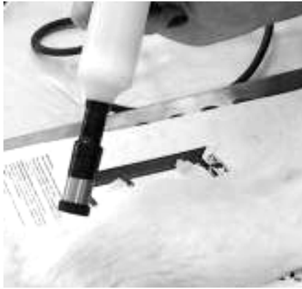
Fig. 4. Sensitive part of the gamma probe protected with a tungsten collimator Source: Author
